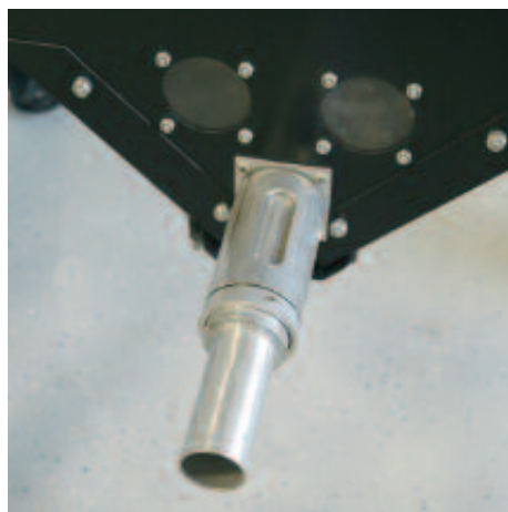
Probe for vacuum take-off.
