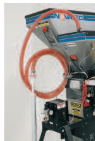
ML Series Venturi Loader for removable hoppers.
