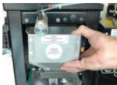
Removing mixing chamber.
